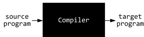
Fig. 1. At the highest level, a compiler is interpreted as being a black box with an input, and output, and an opaque implementation.
